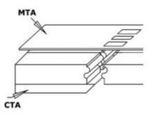
**PREF A - TO 18:** It forms and cuts 2.54 pitch transistors. It is possible to increase the D measure by spacing the MTA mask
