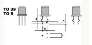
\* The "c" value is referred to boards of 1.5mm thickness
