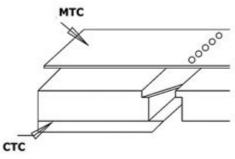
PREF D-LED/CAPACITOR For cutting leds and capacitors when polarity needs to be distinguished. It is possible to increase the C measure by spacing the MTC mask
