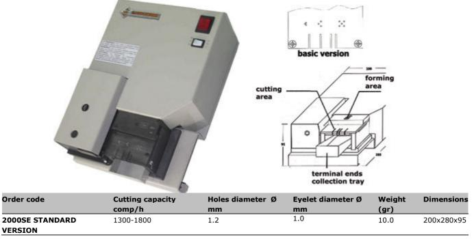
2000SE is a pneumatic machine for the forming and cutting (standard height 3 mm) of untaped electronic component terminals. 2000SE is supplied with a further cutting mask (1.5 mm height).
