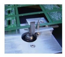
Two tool holding blocks are provided with the R100. The first holds a flat guide blade which is designed to make it easy to route the tabs from a rectangular panel. The second provides 3 adjustable guide pins which can be set for any size round panel. Standard guide pins or guide blades are provided for 0.125", 0.092" and 0.062" routed sections.
