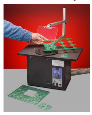
Safely singulate PCB panels by finish routing tabs.
